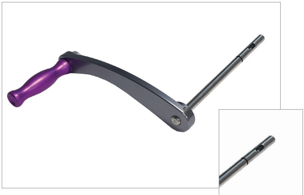
KYRA Curve Crank Handle KYRA9010 Rotational handle for the Curve Spine Frame to create lordosis. Machined marked and windowed to help ensure positive connection with the Curve Spine Frame.
